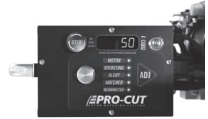
DRO computer in READY mode displaying speed.
