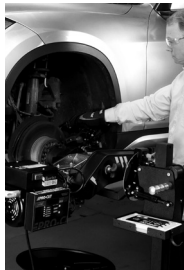
STEP 4. Technician sets cut depth.
