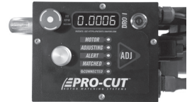
DRO computer compensated for lateral run-out to 0.0006" and ready to cut.
