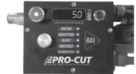
DRO computer in READY mode displaying speed.
