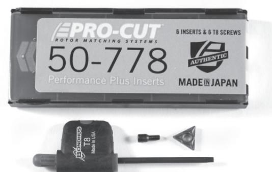
The maximum recommended depth of cut is 0.015" / 0.38mm per insert.
