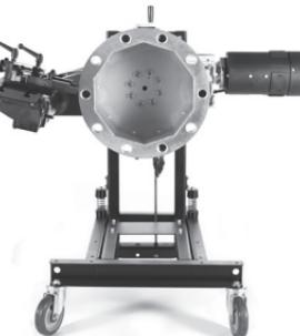
Step 2: Mount the adapter to the lathe with the 8 included bolts
