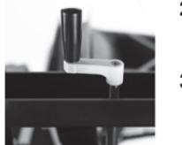
Use crank handle to fine adjust height of lathe once height of vehicle is set.
