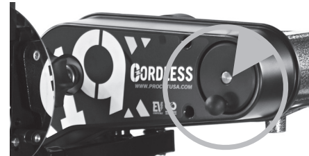
Move the cutting head by turning the clutch knob shown above, clockwise for away from the rotor, counter-clockwise for towards the rotor.
