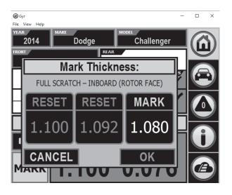
14e. The remaining material that can be removed will be displayed in the lower right hand corner of the screen.
