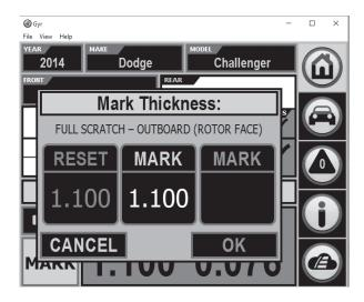
14c. Rotate the other dial knob to bring the back cutting arm in until it scores a complete circle on the back side, then press the right Mark button.
