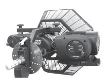
Lathe in upside-down position. You will need to flip the lathe over into this position to machine one side of the vehicle if there is a dust shield, or other interference behind the rotor.
