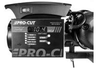
This value represents hours and tenths of an hour that the motor has to run.
