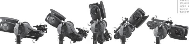
After loosening the trolley handle, the lathe can be flipped over to machine the opposite side of the vehicle.
