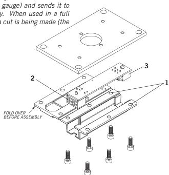
Remove the cover on the bottom of the bevel gearbox assembly. Replace it with the 50-1148 assembly. taking care to aim the eight pin connector towards the lathe body. With the lathe unplugged from AC power, seat the 6 pin connector from the slide sensor, and the 8 pin connector from the lathe's harness. These are waterproof connectors and they seat firmly. Please make sure the small catch latches over the post on the top of each connector to ensure a complete connection. Re-power the lathe.
