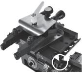
Set the shut-off cam (circled) by loosening the thumbscrew and positioning on the rail so that the cam will depress the stop button when the cutting tips clear the rotor.
