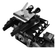
Detail of the gib adjustment screws
