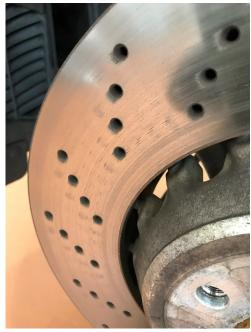
"Trailing marks" may be visible from the crossdrilled holes after resurfacing. They are the small dark spots adjacent to some of the existing vent hole drillings.
