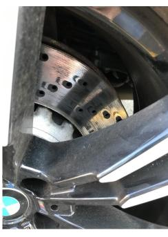
The customer should be made aware that the trailing marks will become more visible with brake applications and will eventually disappear with normal driving.
