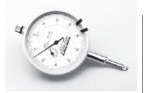
\*NOTE: The Dial Indicator (above) is essential in troubleshooting compensating issues with the Pro-Cut on-car lathe. I recommend the following tools for servicing Pro-Cut on-car lathes. —JOE G.
