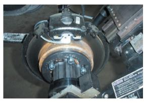
2004 and up **Dodge Caravans** with the rear disc brakes now have the caliper mounted at 12:00 on the rotor. The front of the Caravan still has the forward positioning of the caliper which allows for a cut with no problem.
