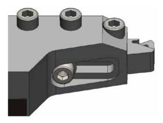
The cutting arm reaches 77 mm (3") in the shortest position
