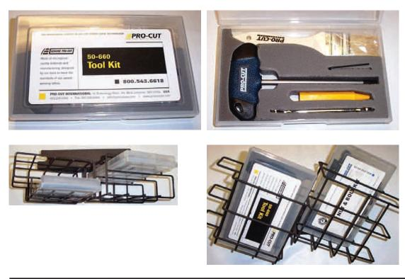
The **50-660 Tool Box Assembly Kit** is standard issue with any new lathe package. The kits are also available separately.
