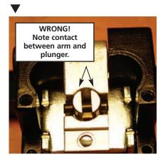
**INDICATION:** If the Solenoid "clicks" loudly then progressively clicks softly after the part has been cleaned and rebuilt. This procedure is for the **50-100 "Black"** Solenoid only.
