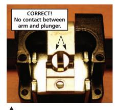
Figures 1/2. Correct solenoid adjustment should always have clearance between 50-102 striker arm and plunger for the entire travel of the plunger.
