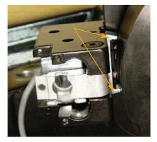
Figures 5. Both ends of 50-103 striker arm must be touching the side of the flange when assembled properly.
