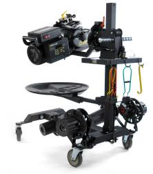
Pro-Cut's PFM 9.2DRO on-car brake lathe
