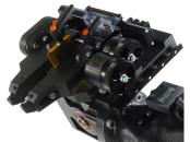
**G2X Cutting Head (50-1200)** slide, center, lock and set lock handles. Simple operation and visibility of the control knobs as they are facing the technician. This cutting head will also measure the thickness of the rotor before, during and after the cut.
