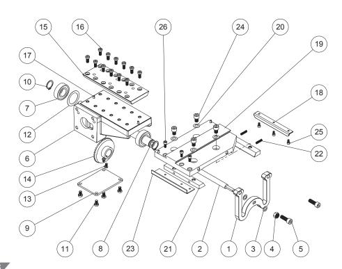
X9 PARTS DIAGRAM PRO-CUT 50-2195 TROLLEY 60 PART NUMBER 50-2047 (32)(12) (16) (51) (57)(48)(54)
