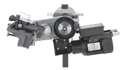
Lathe in upright position. Note that adjustments to cutting head are made in this position.
