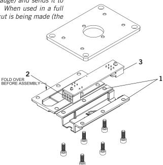
Remove the cover on the bottom of the bevel gearbox assembly. Replace it with the 50-1148 assembly, taking care to aim the eight pin connector towards the lathe body. With the lathe unplugged from AC power, seat the 6 pin connector from the slide sensor, and the 8 pin connector from the lathe's harness. These are waterproof connectors and they seat firmly. Please make sure the small catch latches over the post on the top of each connector to ensure a complete connection. Re-power the lathe.
